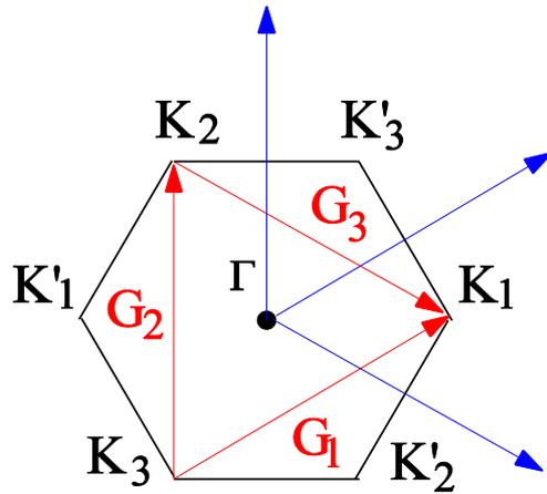
$$G_1 = \frac{2\pi}{3L} (3, \sqrt{3}), \quad G_2 = \frac{2\pi}{3L} (0, 2\sqrt{3}), \quad G_3 = G_1 - G_2$$
